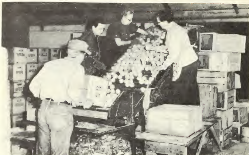
Figure 2.--Hand dumping peaches from field lugs onto the sorting table. Also shown are sorters who remove debris, culls, and overripe fruit.
